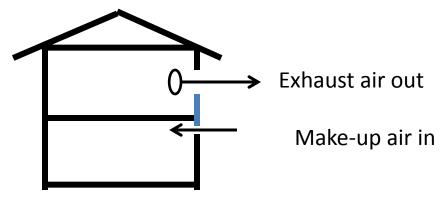
Make-up air is intended to limit the negative pressure in the home during the operation of exhaust devices
