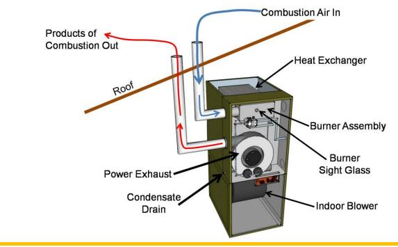
Note: These appliances must be able to function and draft properly at a negative pressure of 50 Pa.
