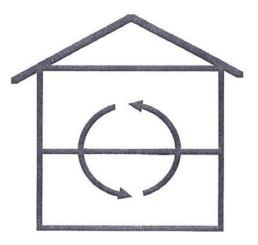
Circulation air is intended to mix the indoor air for improved comfort and to provide more uniform indoor conditions.
