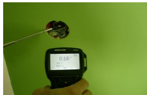
Figure 7: Velocity of air flow measured in a low energy building, left: through the gap between gypsum board of ifloorl, right: elctric socket located in interior wall
