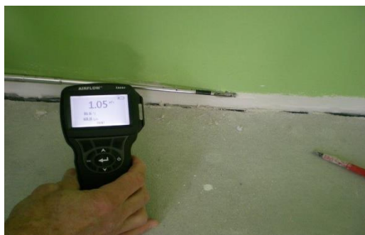
Figure 7: Velocity of air flow measured in a low energy building, left: through the gap between gypsum board of ifloorl, right: elctric socket located in interior wall
