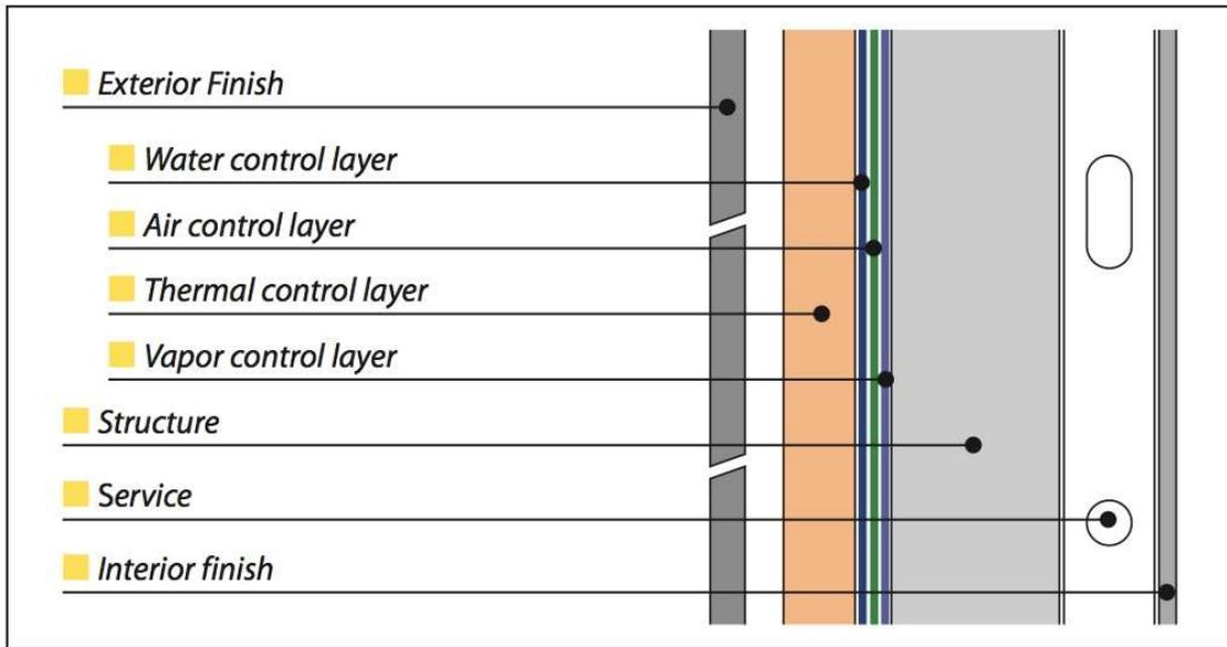
**Figure 1: Diagram of the "Perfect" Wall showing ideal sequence of assembly layers**
