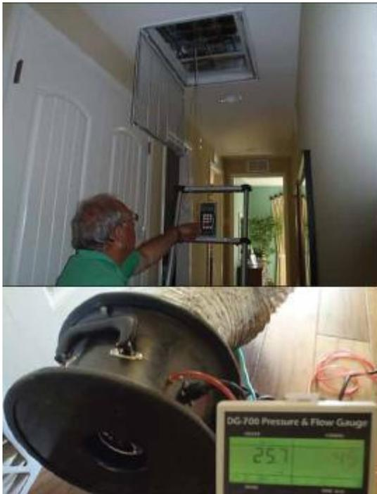
Blower door and leakage testing
